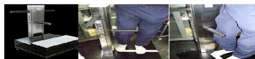
Phot 1. Patented torque meter 1 to measure flexion and extension muscle strengths of both legs in standing posture.
